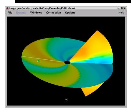
Velocity data from the ENLIL model is interpolated along a radial line in the ecliptic plane and displayed in a second window
