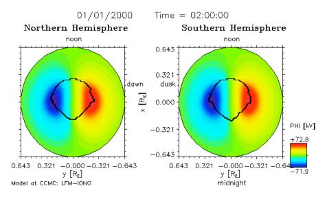
It shows the potential contours (in color) and the open/closed boundary (dark line) in the ionospheres of the model. From the legend scale you can obtain the cross polar cap potential ( $72.8+71.9 \sim 145 \text{ kV}$ ).
