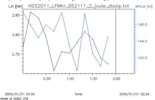
From this, you can get the total cross polar cap potential (144 kV) and the total current (2.72 MA). Use this to fill in part of the table in part 2.
