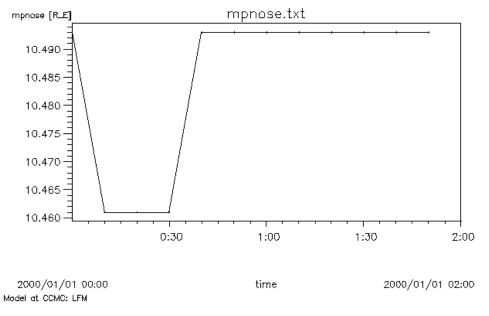
The plot shows the position of the magnetopause as a function of simulation. The standoff distance at the end of this run is  $\sim 10.5$  Re.
